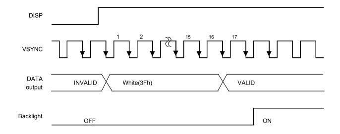
After Display off, "White" data is outputted for 5-Frames first, from the falling edge of the following VSYNC signal. Please turn off the power supply promptly after OFF of "DISP".
